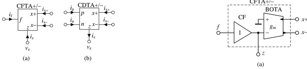
Fig. 1. Circuit symbols of (a) CFTA, (b) CDTA
