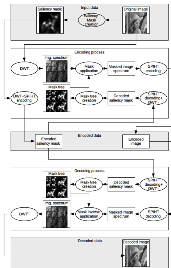
Fig. 1. Schematic picture of whole SM SPIHT encoding and decoding process
