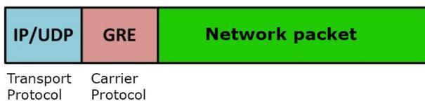
Fig. 5: The structure of encapsulated packet
