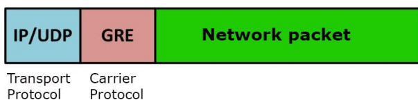
Fig. 6 The structure of encapsulated packet
